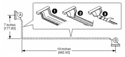
Figure 32: SCSI Cable Length Required
